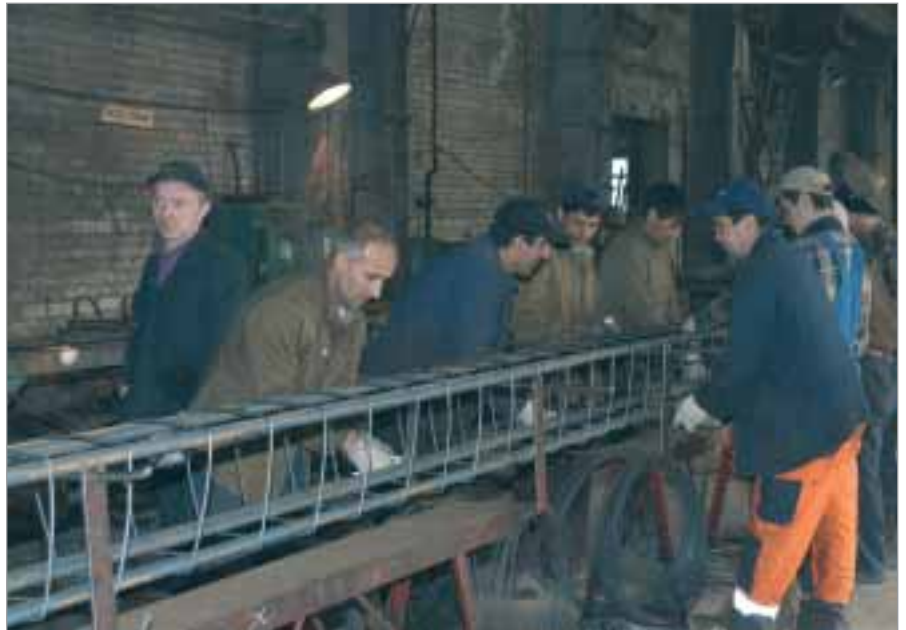
Manual weaving of reinforcement cages at SiB-Center, St. Petersburg
